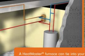
A HeatMaster<sup>ss</sup> furnace can tie into your home heating system very effectively. A water to air heat exchanger can be installed into the existing plenum of your furnace and a water to water heat exchanger can be installed in your domestic water system.
